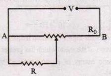
A resistance of R draws current from a potentiometer. The potentiometer wire, AB, has a total resistance of R<sub>o</sub>. A voltage V is supplied to the potentiometer. Derive an expression for the voltage across R when the sliding contact is in the middle of potentiometer wire.
